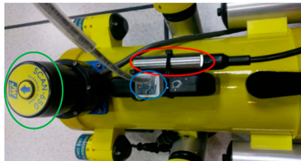
Figure 1. The remotely operated vehicle (ROV) and experimental sensors. The red oval is a water pressure gauge. The blue oval is an inertial measurement unit (IMU) sensor. The green oval is the scanning sonar.
