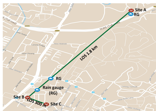
Figure 1. Measurement links map in Kuala Lumpur, Malaysia for 1.8-km and 300-m line-of-sight (LOS) path at 73.5 and 83.5 GHz E-bands between Kolej Siswa Jaya (Site A) and Menara Razak, Universiti Teknologi Malaysia (Site B); and 300-m LOS path at E-band between Site B and Residensi UTM (Site C).
