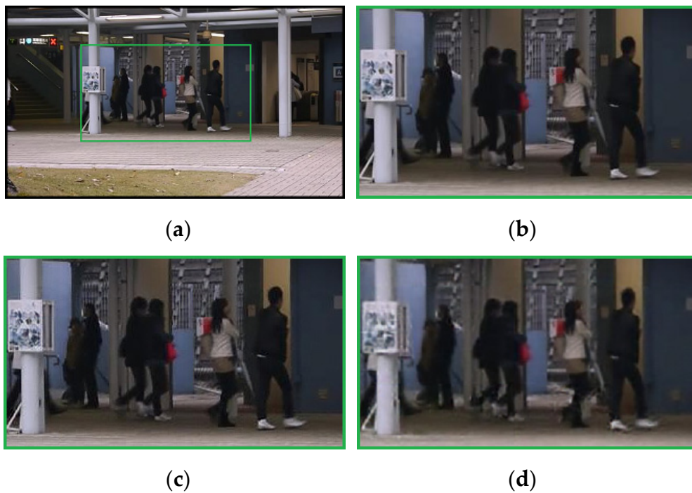
Figure 5. Experimental results on the CUHK dataset. The ground truth is shown in the first row and the generated outputs are shown in the second row: (a) The full ground truth, (b) the ground truth, (c) the output of the proposed method without refinement (PSNR = 32.87, SSIM = 0.935), (d) the output of the proposed method with refinement (PSNR = 31.39, SSIM = 0.914).
