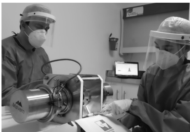
Figure A2. The experimental setting with the clinician in the left side of the image, the measurement device, Insitac S (Malvern Panalytical Ltd., Malvern, UK) in the middle, the dental assistant holding the high-volume evacuator in the right and the real-time analytical computer equipment in the background.
