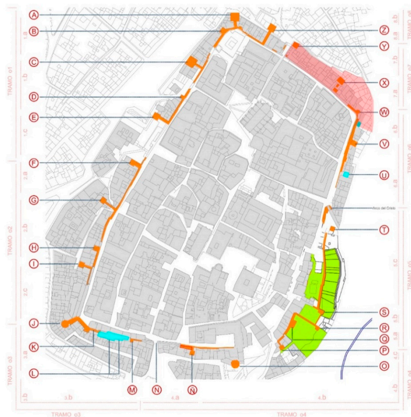
Figure 1. Location map of the intervention. A—garbage tower; B—Spain arch street tower; C—Bujaco tower; D—pulpit tower; E—Yerba tower; F—oven tower; G—Postigo tower of Santa Ana; H—tower of Calle Adarve del Padre Rosalío; I—Aver tower; J—octagonal tower; K—tower for private use; L—hidden towers (historically located); M—Cornudillas Street tower; N—Mérida gate tower; Ñ—Torremochada street tower; O—Torre mochadi; P—Hernando Pizarro street tower; Q—Covacha tower; R—tower of the cisterns; S—water well tower; T—river tower; U—southern tower of Caleros Street; V—Caleros tower; W—round tower; X—air tower; Y—relief tower; Z—king’s tower.
