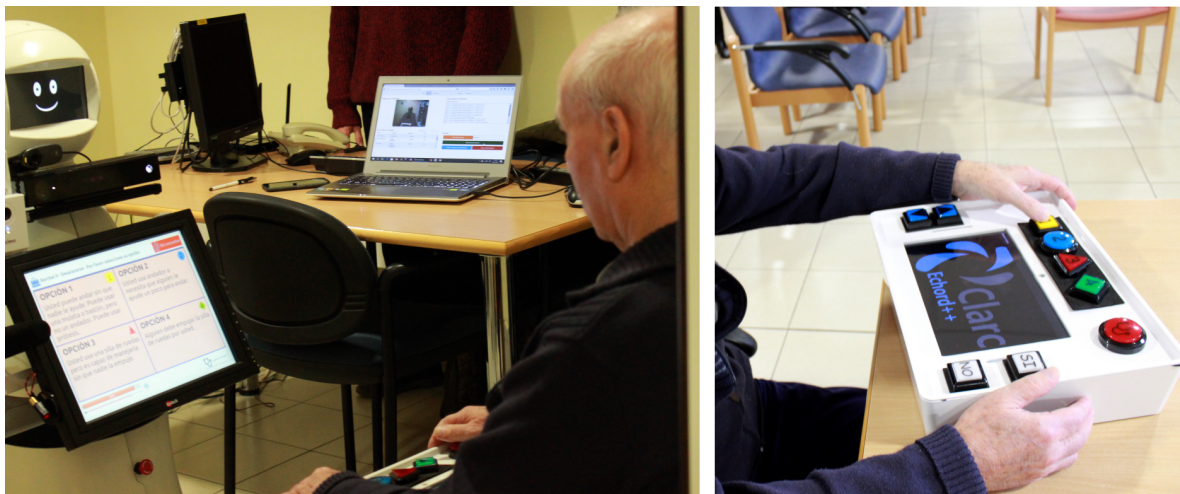
Figure 1. (Left) CLARC interacting with a patient for performing a Barthel test. (Right) The external remote control.
