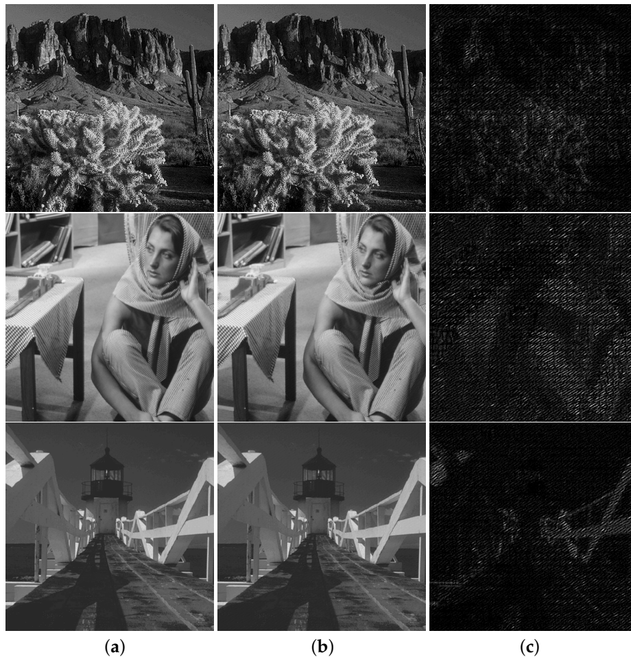
Figure 3. Examples showing invisibility: (a) host images, (b) watermarked images, and (c) magnified difference image, peak-signal-to-noise-ratios (PSNRs) of the first, second, and third row are 37.46 dB, 40.87 dB, and 42.13 dB, respectively.
