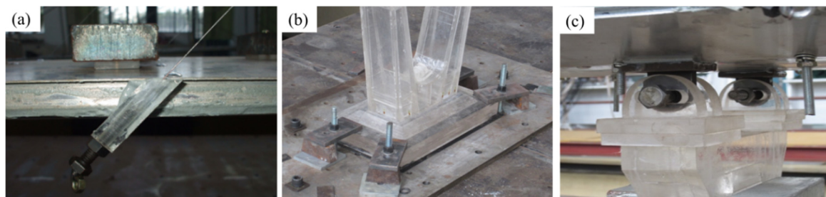
Figure 5. Assembling of the components (a) cable anchor; (b) fixed tower foundation platform; (c) sliding bearing.
