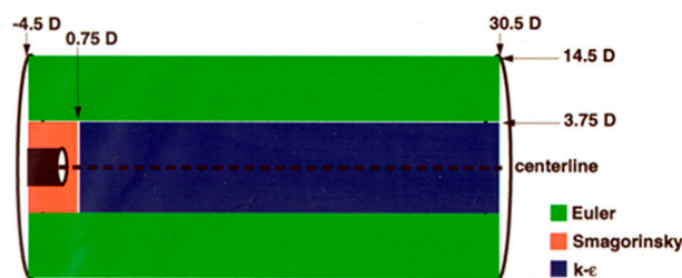
Figure 17. Very large-eddy simulation. Zones of the governing equation (Ref. [58,62]).
