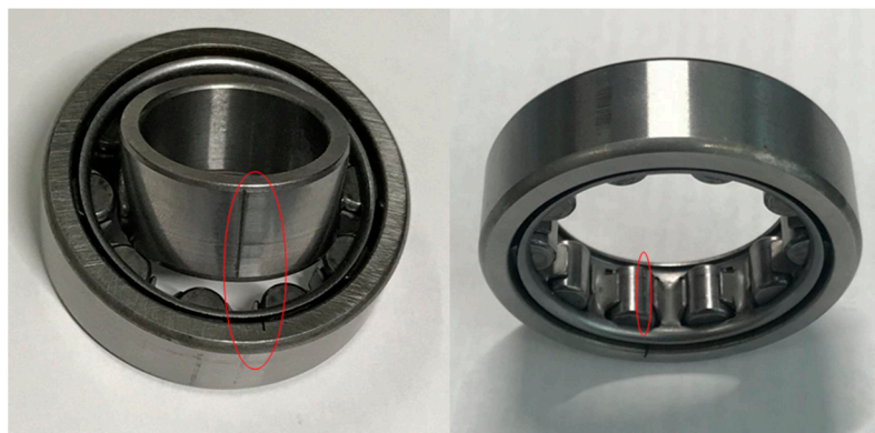
Figure 6. The fault bearing, with defects in (left) inner and our race, (right) rolling element.
