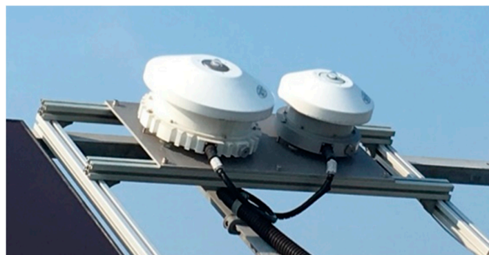
Figure 2. Spectro-radiometers installed at the University of Miyazaki.
