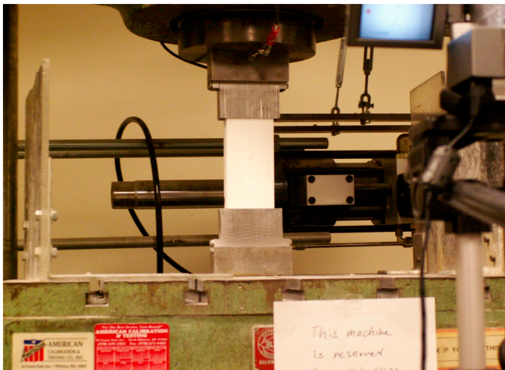
Figure 3. Experimental setup for monotonic and cyclic compression.
