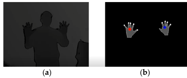
Figure 5. Results of fingertip detection: (a) depth images, (b) fingertip detection.
