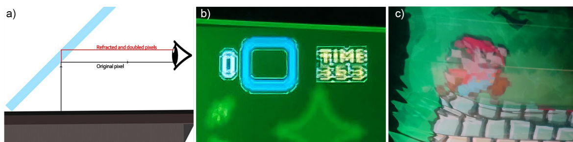
Figure 4. (a) Double reflections ray diagram. (b) Double reflection effect on a 2-mm PE sheet. (c) Wobbly effect on a 0.25-mm acetate sheet.
