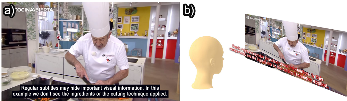
Figure 15. (a) Traditional subtitles on a regular screen. (b) Using SliceView to render subtitles at different depths, enabling the user to change the focal point to reveal partially occluded areas.
