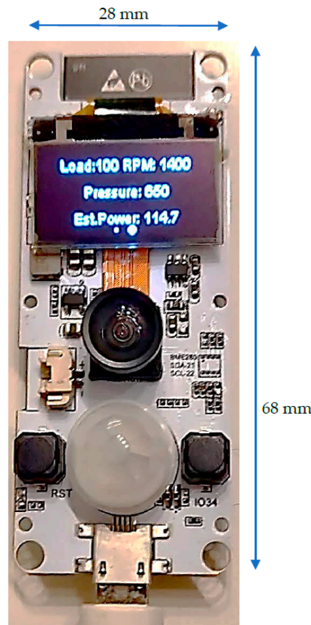
Figure 15. “AI in a nutshell” solution with an effective power ( P_e ) = 114.7 kW computed by the embedded ANN for load = 100%, speed = 1400 rpm, and pressure p = 650 mmWC.
