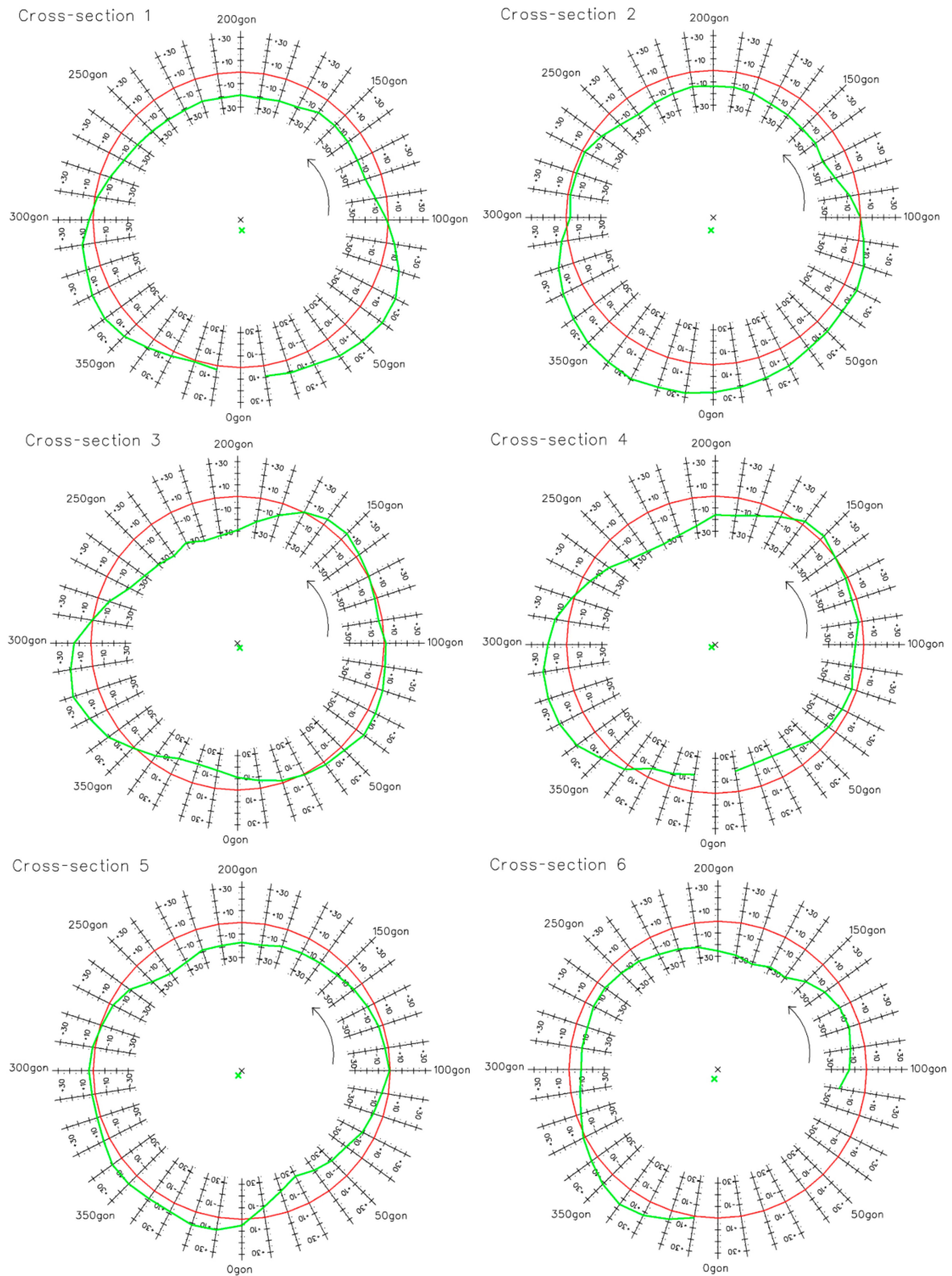
Figure 31. The selected cross-sections of the RK shell. Linear units of the ovality [mm].
