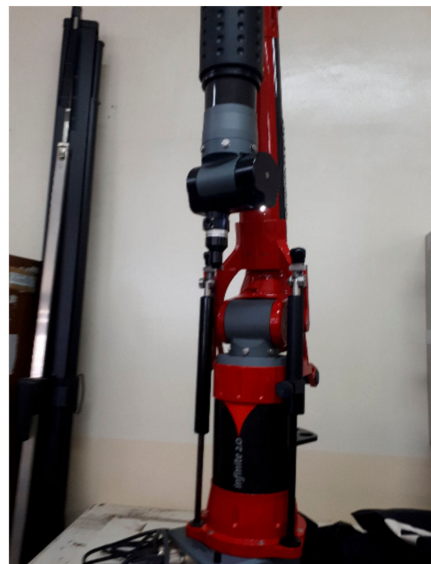
Figure 6. Cimcore® Infinite® 2.0 Portable coordinate-measurement machine (CMM).
