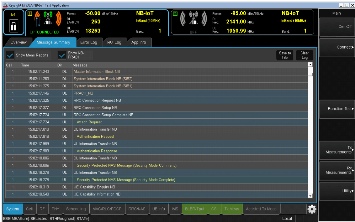
Figure 8. Control messages between the UE and the eNodeB emulator.
