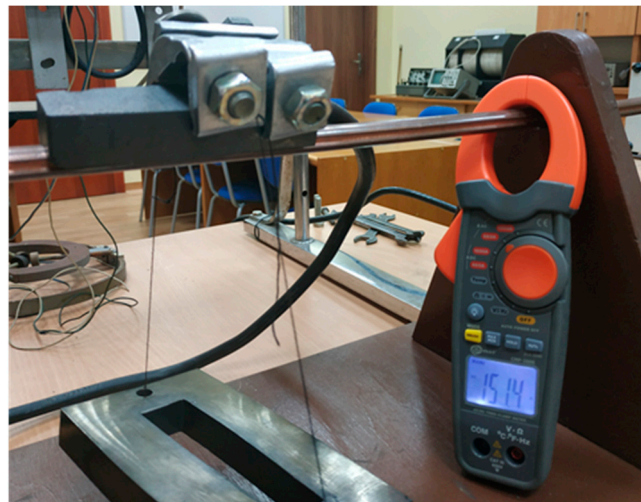
Figure 4. A photograph of the laboratory stand for testing current ampacity.
