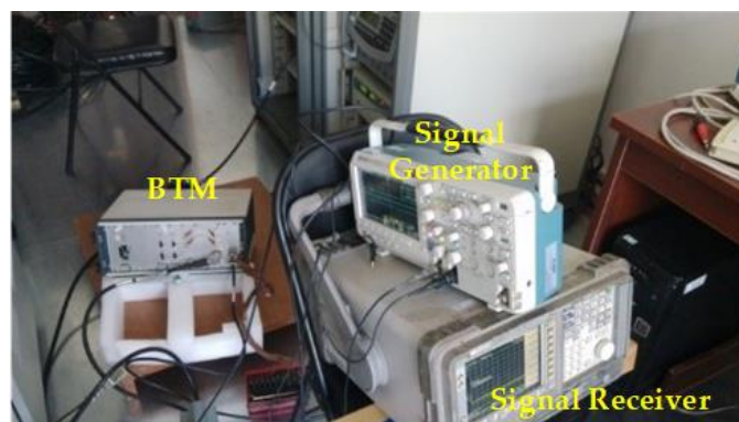
Figure 13. The setup of the test for getting h .
