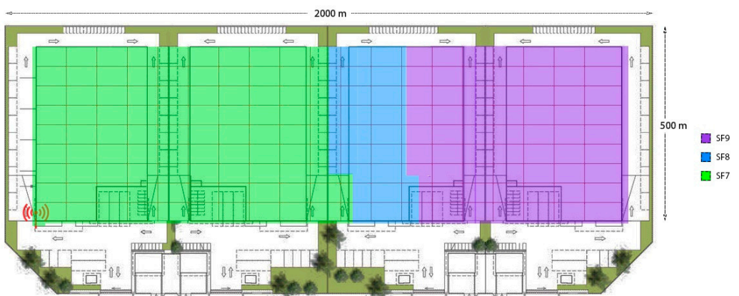
Figure 10. Results of SF for downlink traffic configured in every node at the end of the simulation, overlaid on the site map.
