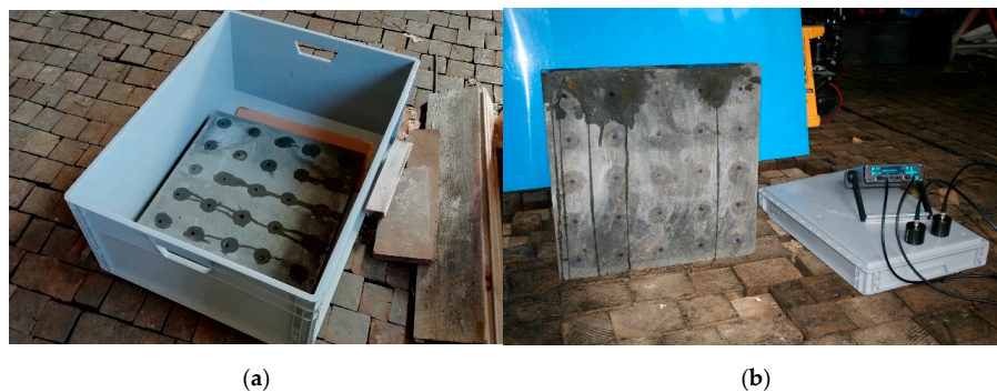
Figure 5. Testing of the influence of rainwater on the results of the measurement using the ultrasonic method. (a) The V3 slab in container, prepared for rainfall simulation, (b) the V3 slab measurements.
