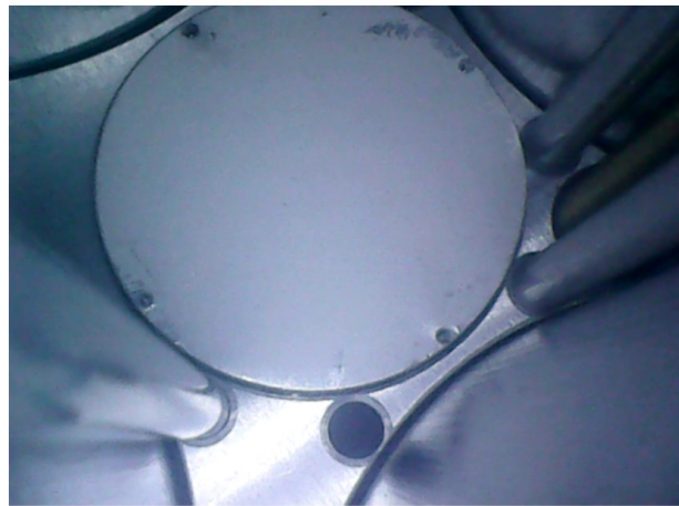
Figure 3. Circular scintillating screen (23.8 mm diameter, total thickness about 2 \mu\text{m} ) illuminated by the LED of the endoscope camera. The perspective angle is corrected by the pre-processing software.
