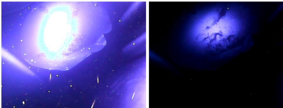
Figure 5. 2D images taken by the \pi^3 detector with beam currents of 360 nA (left) and 60 nA (right).
