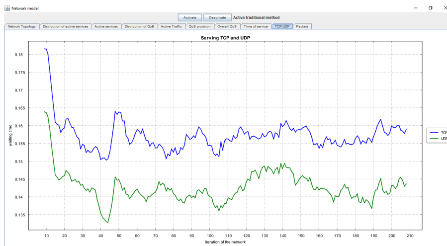
Figure 31. The average waiting time for TCP/UDP (Transmission Control Protocol, User Datagram Protocol) services using the traditional method.
