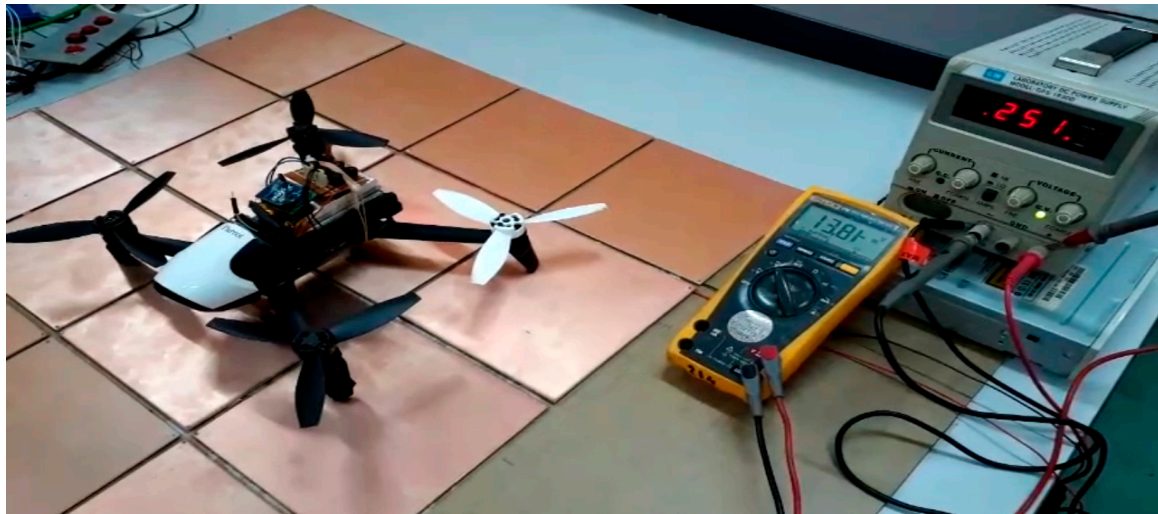
Figure 2. Lab test for the configuration of the chess pad charging platform.
