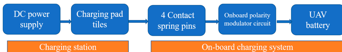
Figure 1. Main system components of the presented charging platform. UAV: unmanned aerial vehicle.
