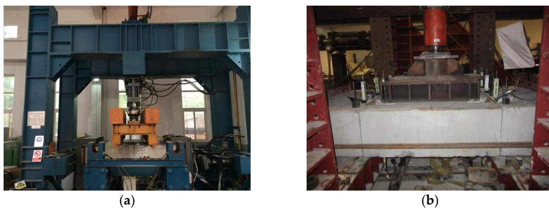
Figure 7. Joint experiments: (a) bending moment resistance experiment; (b) shear resistance experiment.
