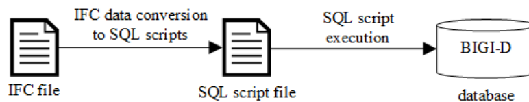
Figure 2. General scheme of importing IFC data into the database. SQL: Structured Query Language.
