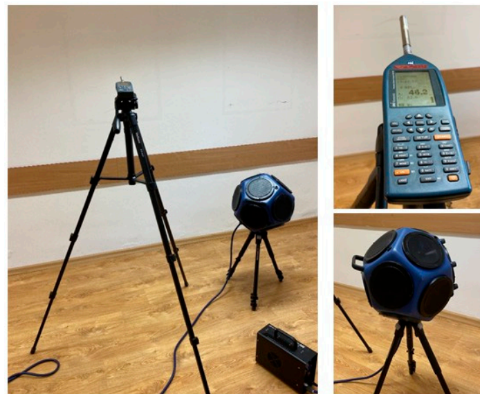
Figure 1. Measuring point and measuring equipment (sound source, microphone).
