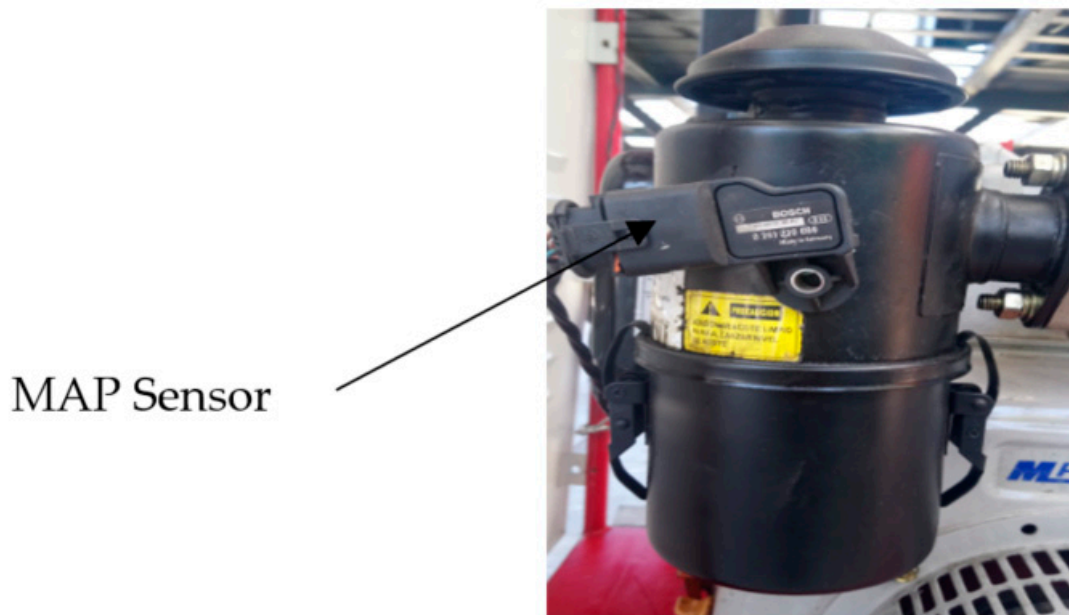
Figure 3. Air pressure sensor placed in the engine air filter.
