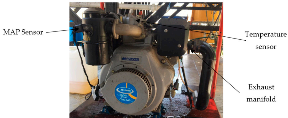
Figure 1. Mpower cylindrical mono diesel engine.
