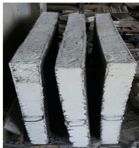
(b) Concreting, curing and staining with white
