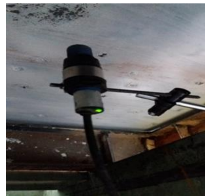
(c) LVDT at the central point below the specimen
