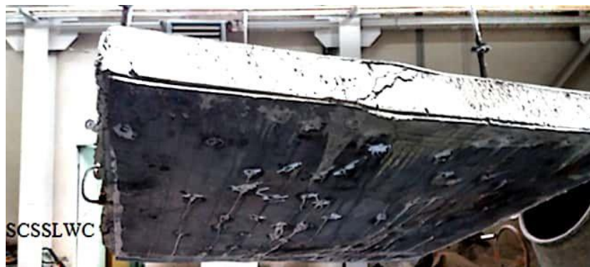
Figure 11. Deformation of the bottom and top plate.
