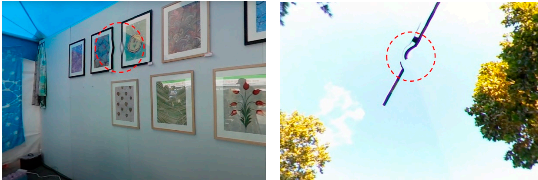
Figure 2. Errors of stitching in a 360° video.
