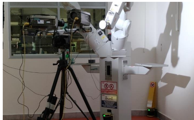
Figure 15. Measurement of IRB1200 by DIC Q-450 system.
