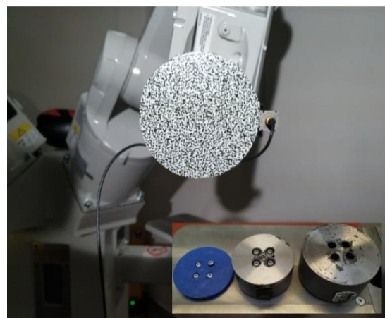
Figure 2. Robot payload with applied black-and-white speckle pattern.
