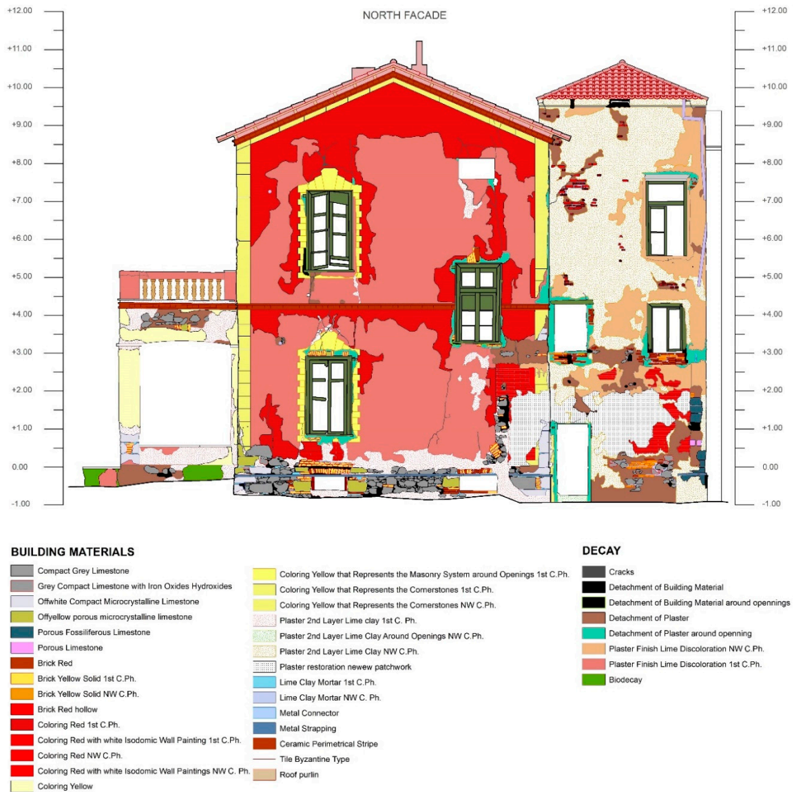
Figure 11. Thematic map of building materials and decay of the north façade.
