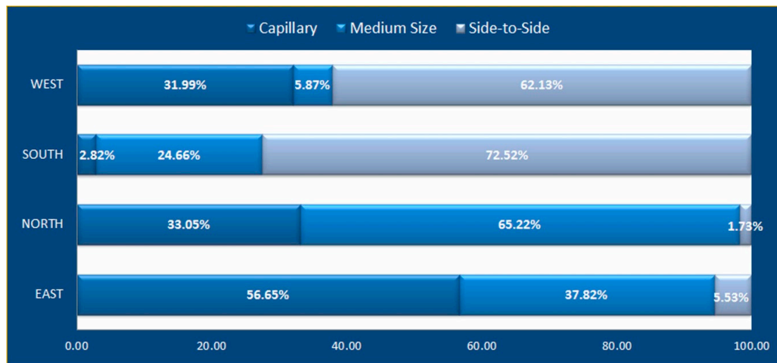
Figure 21. Diagram illustrating the percentage of the length of each type of crack (m) for all facades of the building.
