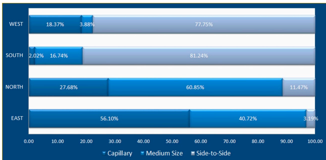
Figure 22. Diagram illustrating the percentage of the area (m 2 ) each type of crack possesses for all facades of the building.
