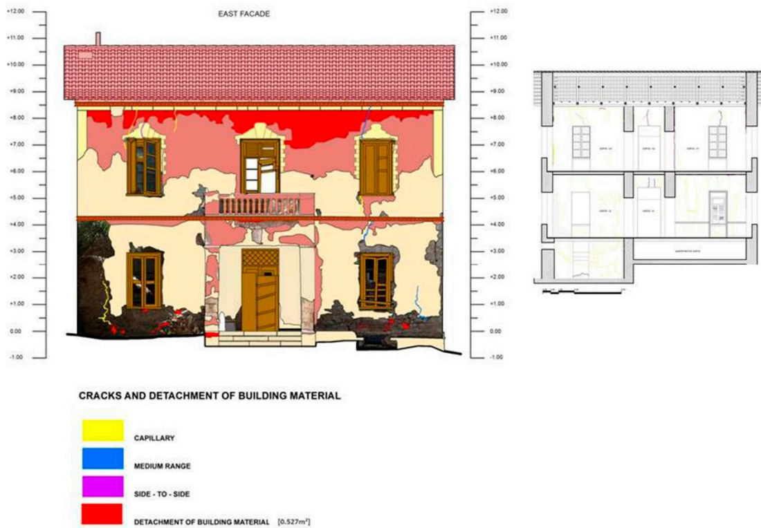
Figure 14. Thematic map of cracks and detachment of building materials depicted on the east façade of the building.
