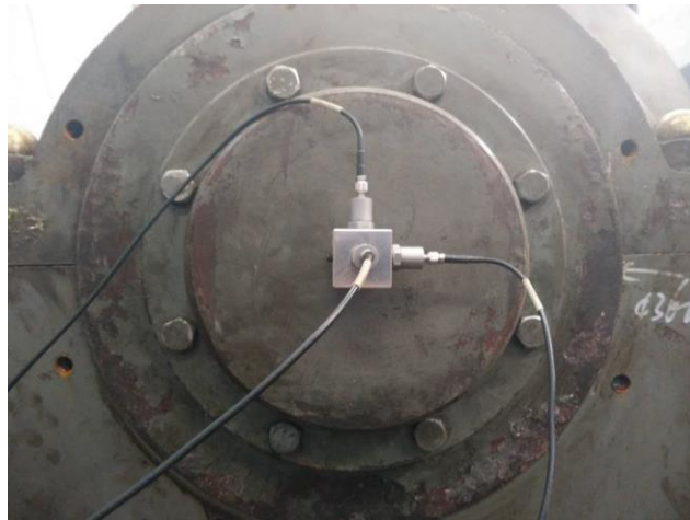
Figure 10. Picture of the mounted vibration acceleration sensor.
