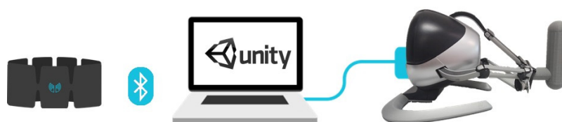
Figure 1. Scheduled illustration of the upper limb rehabilitation platform: Myo Gesture armband (left object in image) and Novint Falcon device (right object in image).
