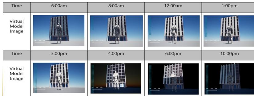
**Figure 16.** Virtual Reality Model Reflecting Changes in Motion in Relation to Daylight at Different Times of the Day.
