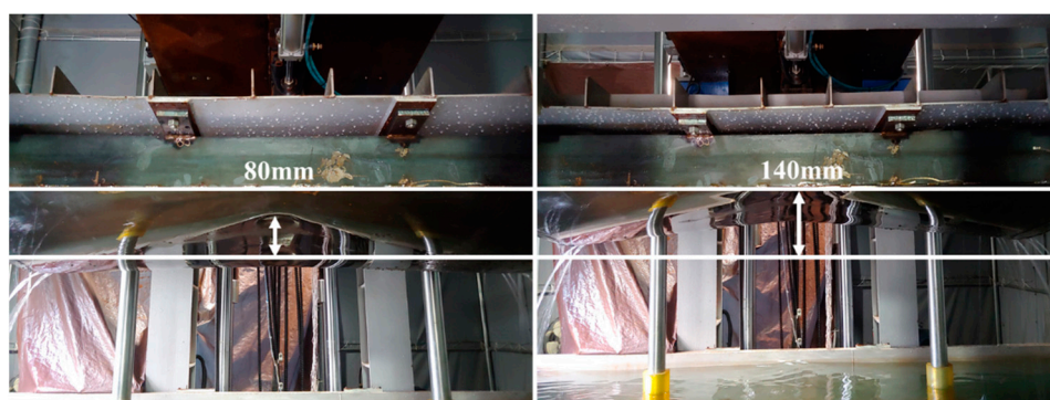
Figure 19. Measurement of the 1st free drop test (left) and the 5th free drop test (right).
