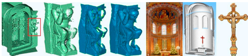
Figure 5. Generation of small complex objects of the cathedral using the meshing function in Geomagic for the segmented point clouds.
