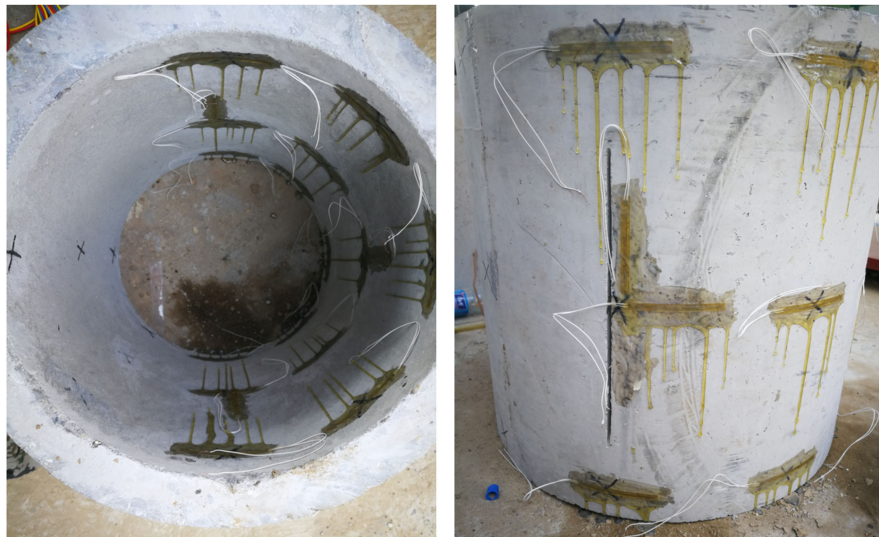
Figure 7. Gluing strain gages in position.
