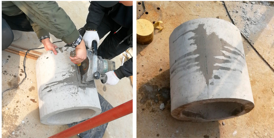
Figure 5. Cutting and forming cracks on the concrete pipe.
