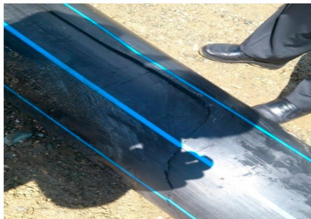
Figure 25. Brittle crack of pipe (photo Scarlatescu).
