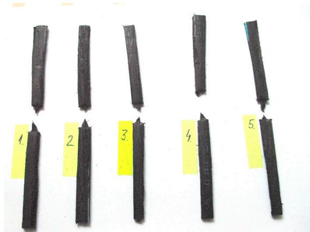
Figure 8. Samples of HDPE pipe  $\Phi 90 \times 6$  broken at traction.
