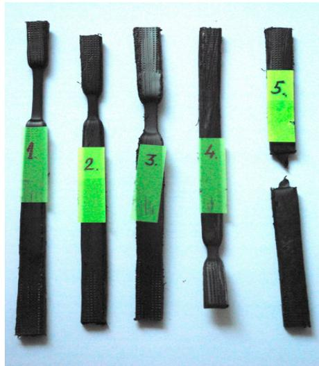
Figure 5. Specimens after traction test.
