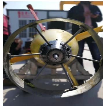
(b) Actuator spindle bending failure
