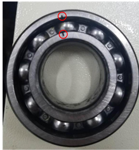
Figure 19. Experimental bearing with multiple faults on the surfaces of the inner race and outer race.
