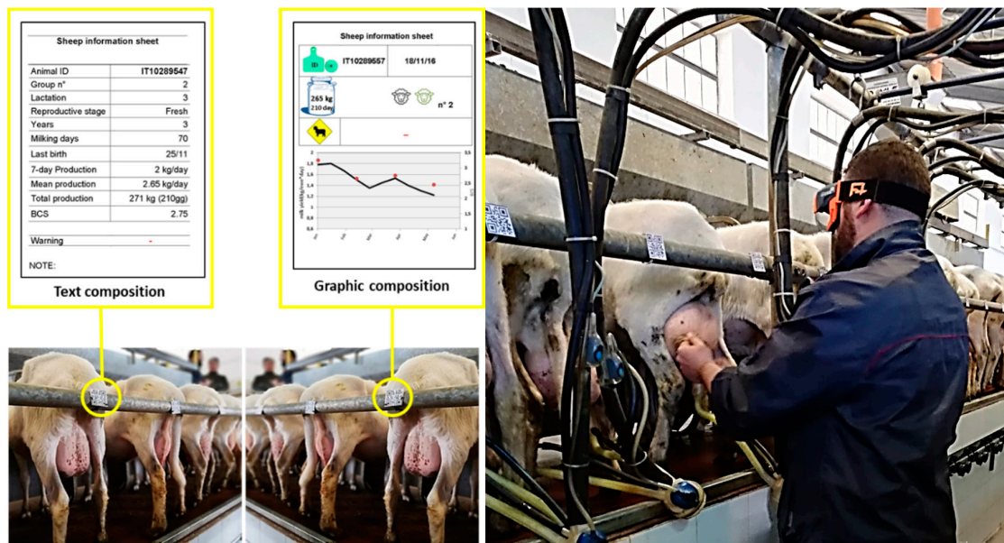
Figure 2. Sheep information sheet text and graphic format (a) and participant reading an animal's information on GlassUp F4 smartglasses (F4SG) while milking (b).
