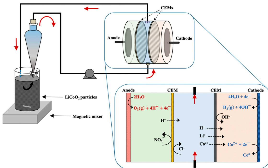
Figure 1. Experimental set-up scheme.
