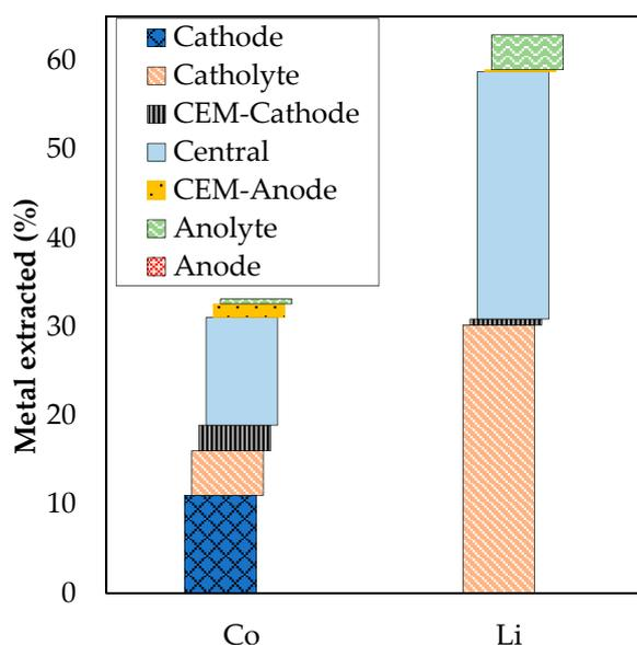
**Figure 5.** Percentage of cobalt and lithium, referred to the total amount of these chemical species in the initial solid samples, in the different parts of the electrodiolytic cell at the end of the experiment.
