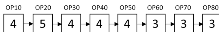
Figure 12. Workcenters arrangement of the production system. The number indicates the amount of machines for each workcenter.
