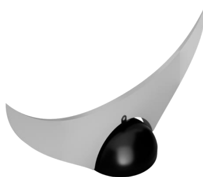
Figure 2. Caudal fin design in Autodesk® Fusion 360™.
