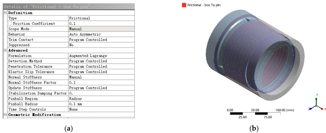
Figure 7. (a) Contact settings and (b) contact surfaces.
