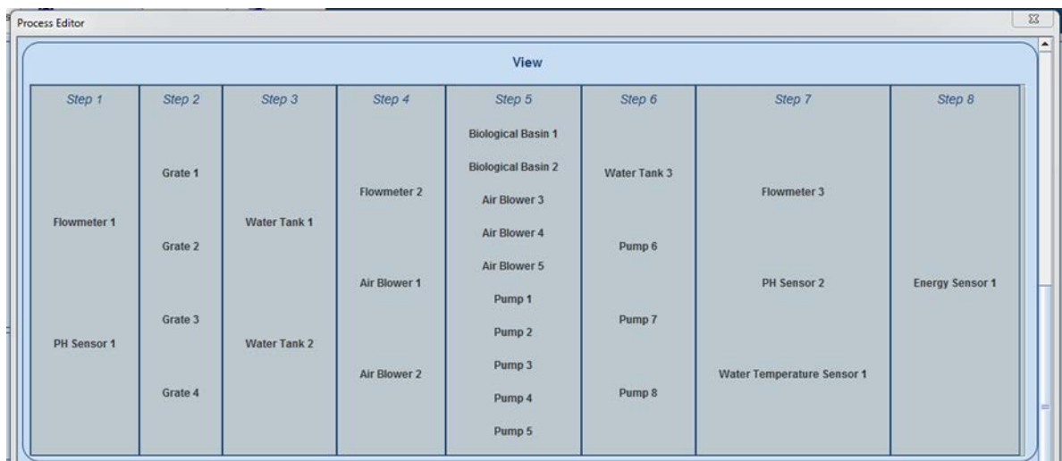
Figure 5. A process of a WWTP, as defined in the Historian Process Editor.
