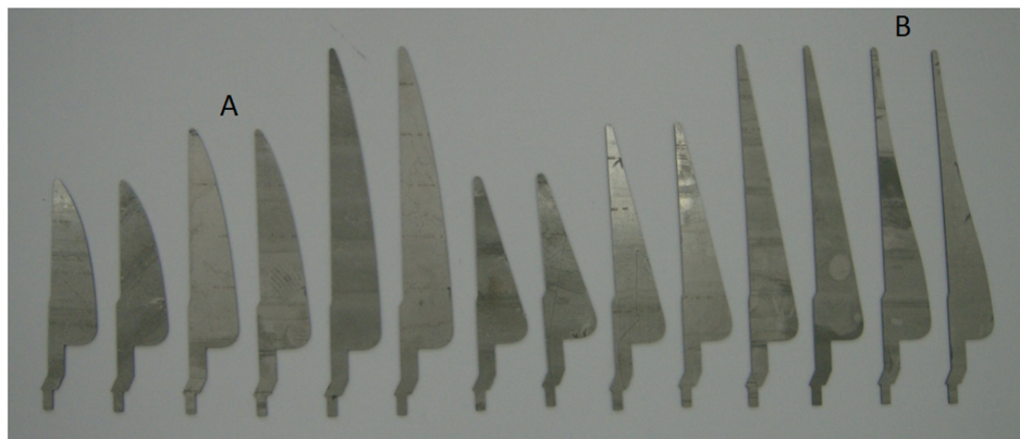
Figure 8. Example shapes of plasma reactor working electrodes.
