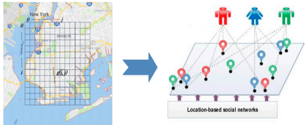
Figure 1. (Left) The whole city graph divided into the CRS i.e., latitude and longitude; and (Right) the LBSN-based driver trajectory as customer pick-up and drop-off. Shaded lines show the driver trajectory, while blue, red, and green nodes show the pick-up/drop-off points.
